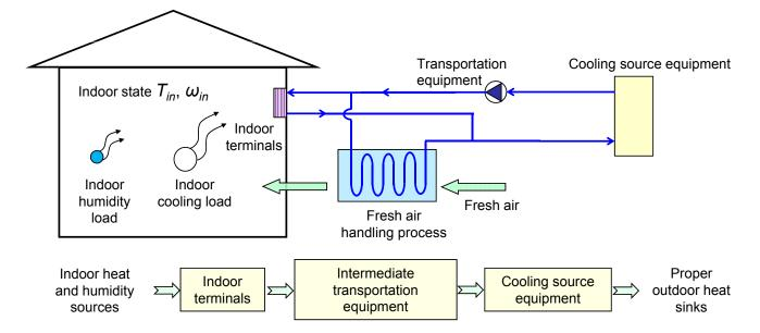
The main processes in an active air conditioning system. This contains a series of processes, including collection, transport and cooling source equipment. Source: EBC Annex 59
