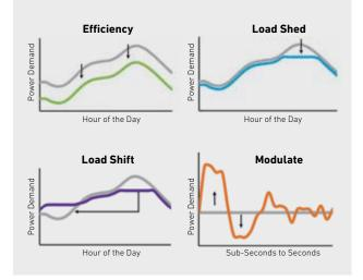
Building flexibility load curves – examples of load curve manipulation. Source: US Department of Energy
