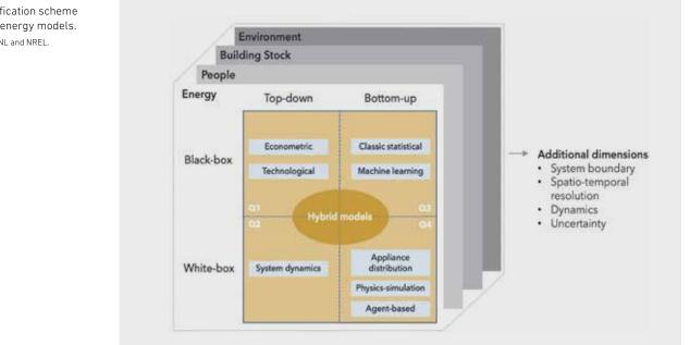
An updated classification scheme for building stock energy models. Source: Courtesy of LBNL and NREL. dealing with bias, guidelines for working towards identifying causal relationships, and systematic approaches to reviewing evidence.
