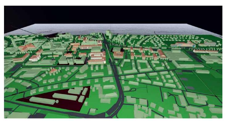
Illustration from a tool in the CHAMPS modelling platform, which highlights building complexes at a community scale that can be simulated for their combined heat, air, moisture and pollutant conditions, including an energy performance assessment. Source: TU Dresden, Germany
